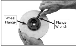
Figure 34. Threading wheel flange onto wheel sleeve.
